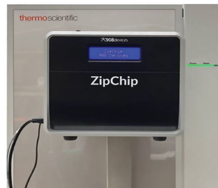
ZipChip mounted to a Thermo Scientific™ Orbitrap 240 mass spectrometer.
