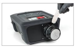
MX908 is equipped with modular accessories for ease of transition between solid and vapor sample types.
