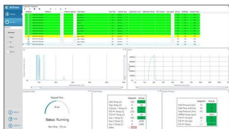
JetStream Acquire User Interface allows real time G908 data acquisition and system status monitoring.
