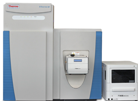
Figure 4: The ZipChip interface and autosampler installed on a Thermo Scientific mass spectrometer.
